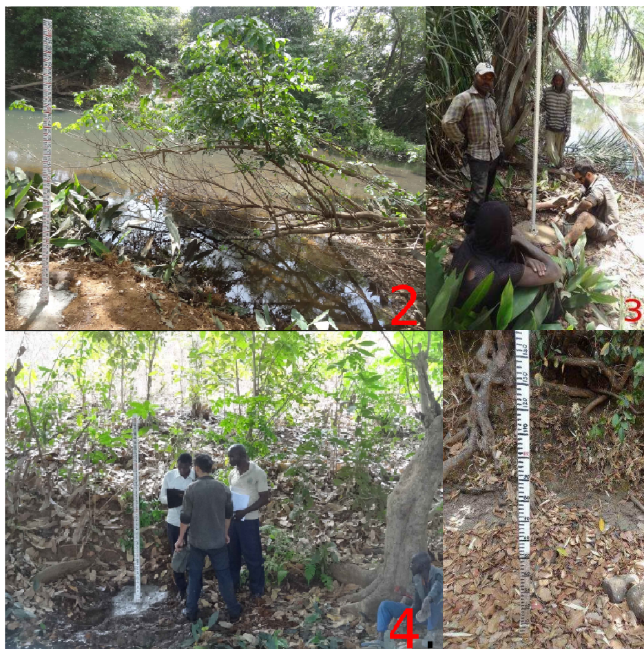
Installation of the scales in Kokoun: 2. Scale placed in Kokouwol river; 3. Scale placed in Bendekourewol river; 4. Team from Kokoun observes the scales and takes data.
